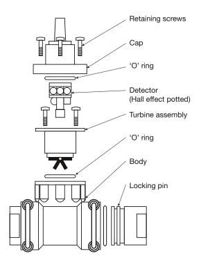
Screws Torque Level = 0.55N-m
