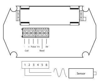
**External power –** Installations with contact closure or magnetic pick-ups can also operate with external power. For powered sensors external power should always be used.
