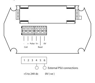
**-NPN pulse i.e. Hall effect sensor.** 2KHz. Max. This input would require external power.
