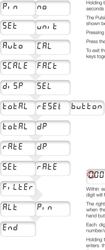
Holding both buttons for a minimum four seconds enters the menu system.
